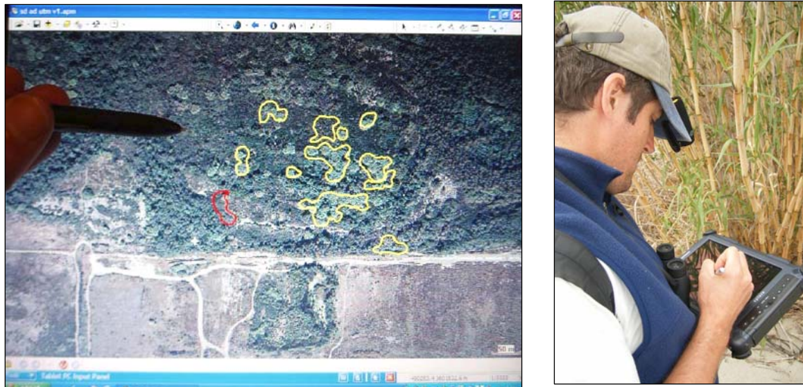
Figure 1 and 2. On-screen digitizing of weed populations using GPS-based Tablet PCs.
