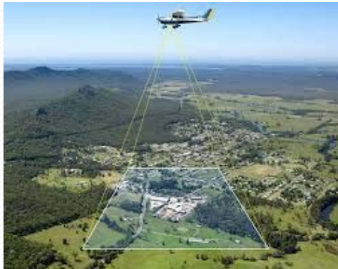
Aerial Photogrammetry With GPS ground Control
